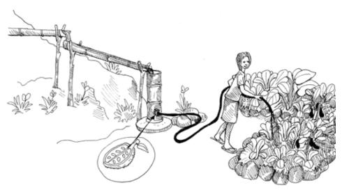
You can also collect water from your house roof or any building large or small, especially those that have a metal sheet roof. You can either buy or make a gutter out of bamboo. Store the water in a tank/s. This water is NOT recommended for drinking as some metal sheets can release lead and other metals into the water, contaminating it.
