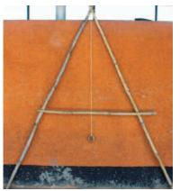
A frame uses gravity only to find level ground
