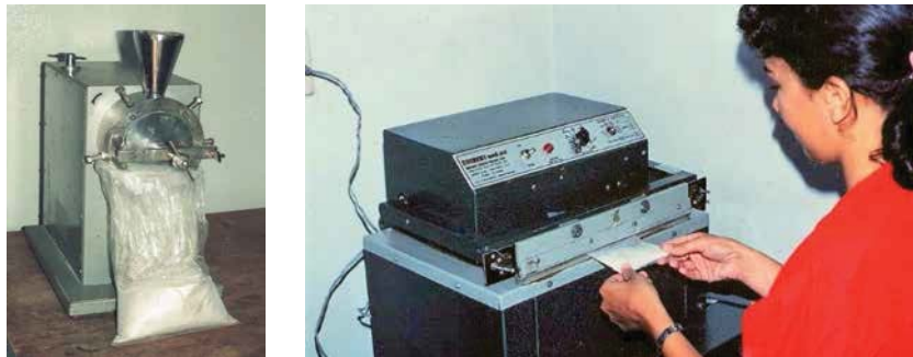
Figure 3. Milling and packaging. Milling of the Baculovirus wettable formulation (left); Baculovirus wettable packaging for application on one hectare of maize crop (right).
